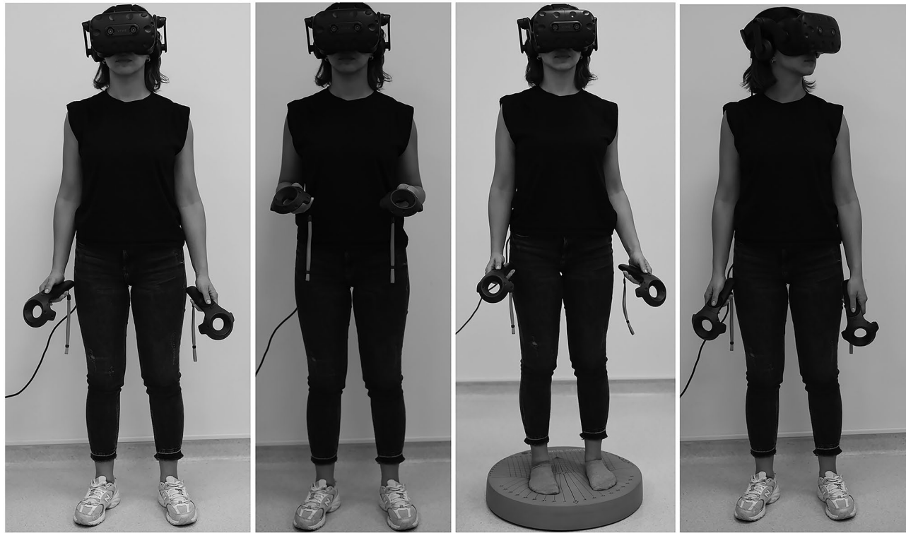
Figure 2. Test conditions: (A) Standing on a firm surface the arm holding the controller at 180 degrees, (B) standing on a firm surface the arm holding the controller at 90 degrees, (C) standing on a foam surface the arm holding the controller at 180 degrees, (D) standing on a firm surface the arm holding the controller at 180 degrees and head turned 45 degrees to the right and left on the yaw axis.
